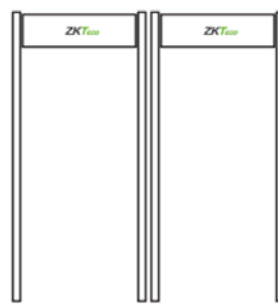
Only need to keep 10cm between two Walk through Metal Detector
